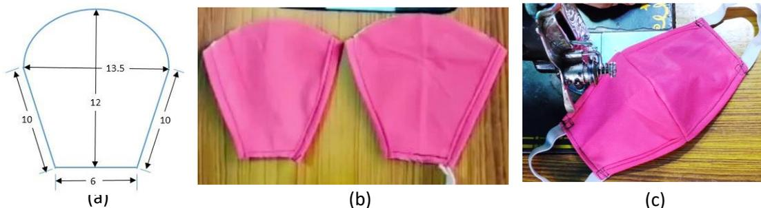
Figure 2: (a) Template of the mask (dimensions in cm), (b) the stitched halves, and (c) the final mask.
