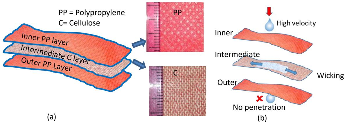
Figure 1: (a) The three-layer structure of the mask, comprising of an innermost polypropylene (PP) layer, an intermediate cellulosic (C) layer and an outermost polypropylene (PP) layer. Insets show the zoomed-in views of the fabrics. (b) Liquid droplet retention in the three-layer fabric.
